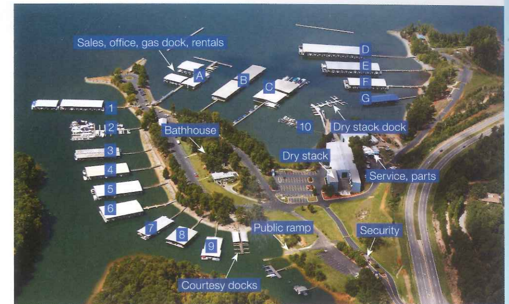
5.8.3 Photo of Gainsville Marina on Lake Lanier, USA, depicting the facilities a marina requires. A–G and 1–10 are docks offering various facilities
