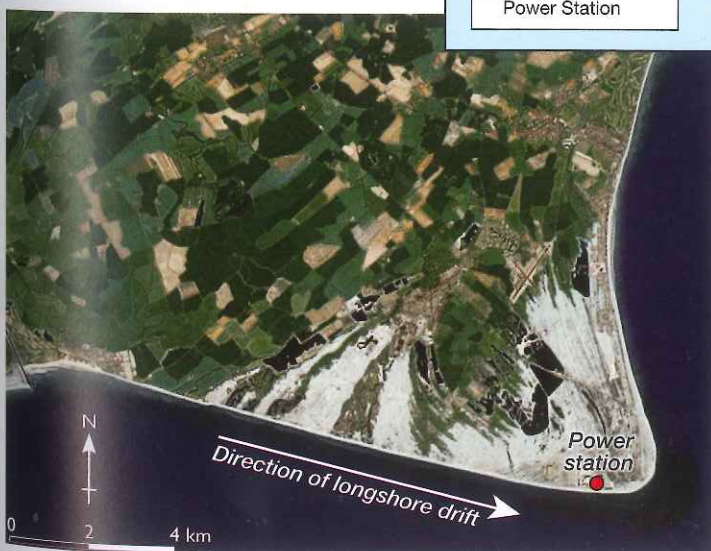
Source 3.8 Longshore drift is threatening Dungeness Nuclear Power Station
